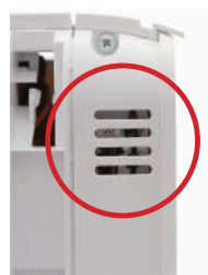
Sensor for indoor temperature and humidity
